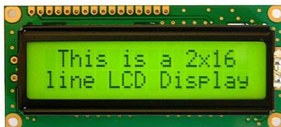
**Gambar 2. 8** LCD 2X16
