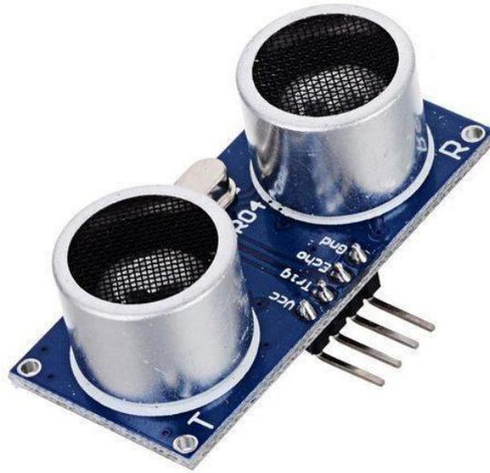
Gambar 2. 8 Sensor Ultrasonik
