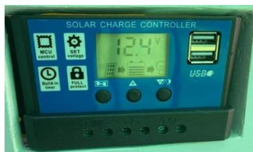
**Gambar 2.7** *Solar charge controller*
