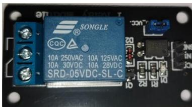
*gambar 2.4 Modul relay 1 channel*
