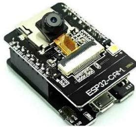
*gambar 2.1 ESP32-CAM*
