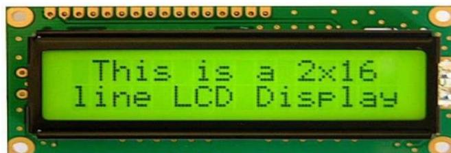
**Gambar 2. 4** LCD 16x2
