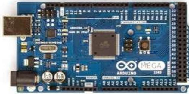
**Gambar 2. 7 Arduino Mega**
