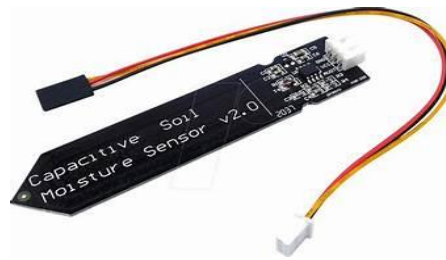
Gambar 2.1 Sensor Kelembaban Kapasitif Sumber: (Effendi, Ramadhani, and Farida 2022).
