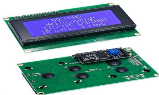
Gambar 2.3 LCD-Display 20x4 I2C
