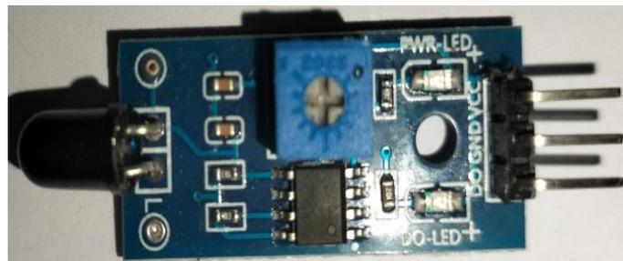
Gambar 2.3 Sensor Api (*Detector Flame*)
