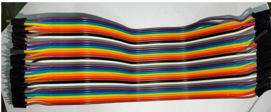
Gambar 2.7 Kabel Jumper *Male To Female*
