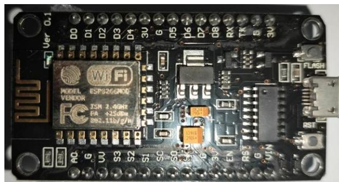
Gambar 2.1 NodeMCU
