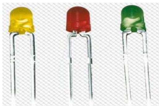
Gambar 2.8 LED ( Light Emitting Diode )
