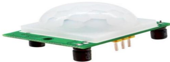
Gambar 2.4 Sensor Passive Infra Red (PIR)
