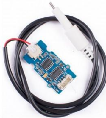
Gambar 2.5 Sensor TDS (Total Dissolved Solids)
