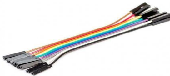
Gambar 2. 11 Kabel Jumper female to female
