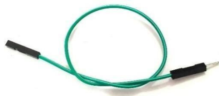
Gambar 2. 9 Kabel Jumper Male to Female
