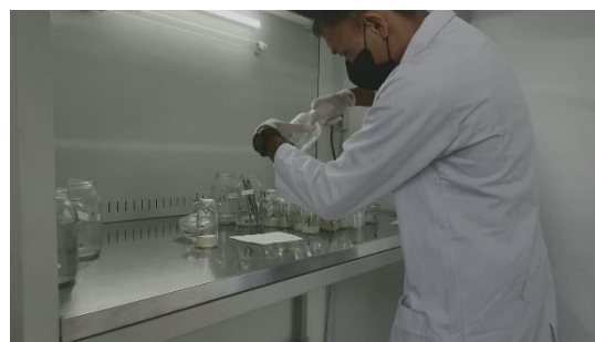
Gambar 1.3 Proses Penanaman Eksplan Di Lamiar Air Flow ( LAF )
