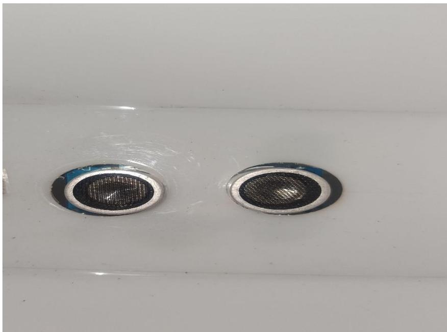
**Gambar 4.4** Tampilan sensor ultrasonik
