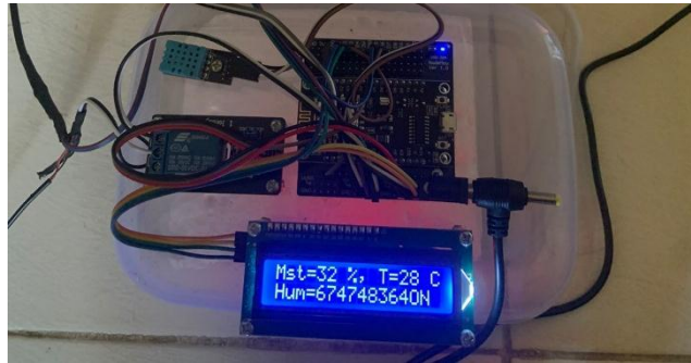
Gambar 4.11 hasil pengujian sensor temperature
