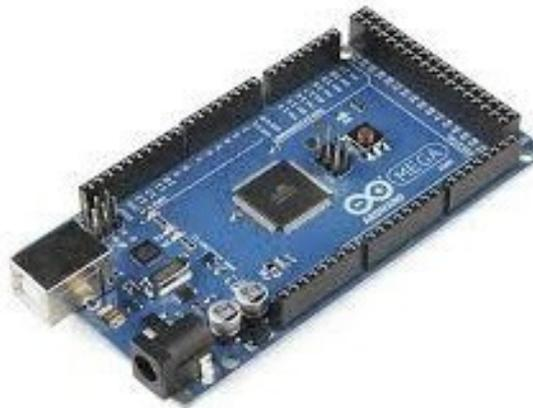
**Gambar 2.2 Arduino Mega**
