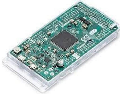
**Gambar 2.5 Arduino Due**
