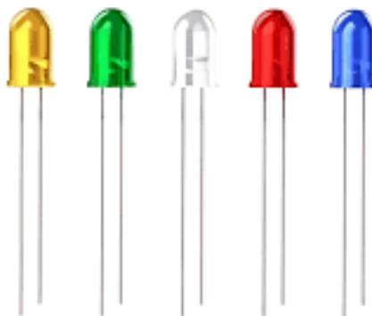
**Gambar 2.11 LED (*Light Emitting Diode*)**
